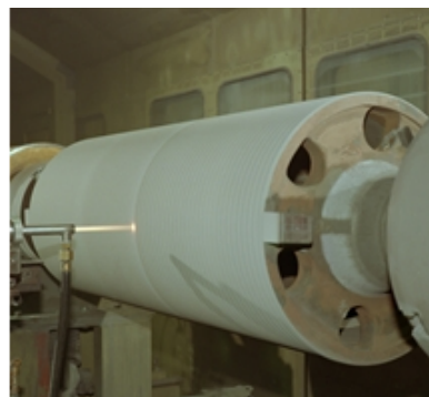
Sink rolls (steel industry, in- sink rolls)
